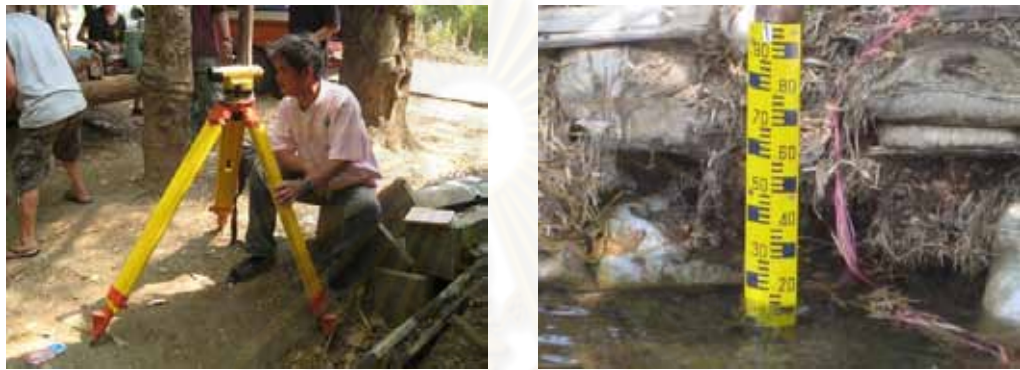
Figure 3-3 Vertical staff gauges setup at Station 1 and Station 4
