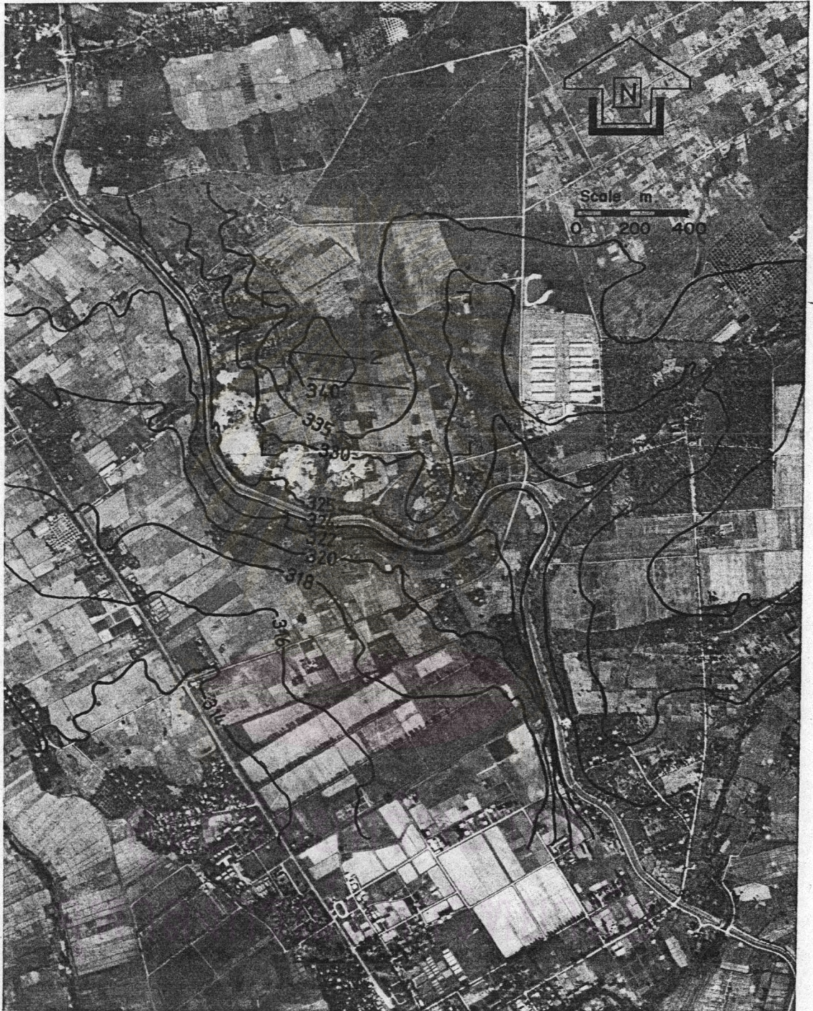
Figure 4-9 Aerial photograph at Ban Huai Kieng area shows the Mae Nam Ping Terrace. Contours are elevation in meter above sea level.
