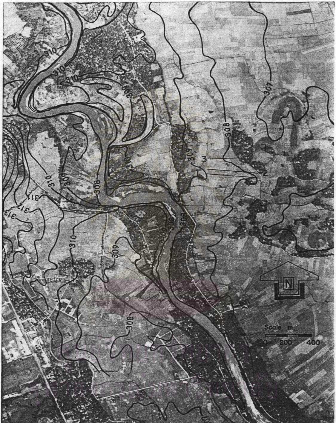
Figure 4-8 Aerial photograph at Ban Rong Wua area shows natural levee. Contours are elevation in meter above sea level.
