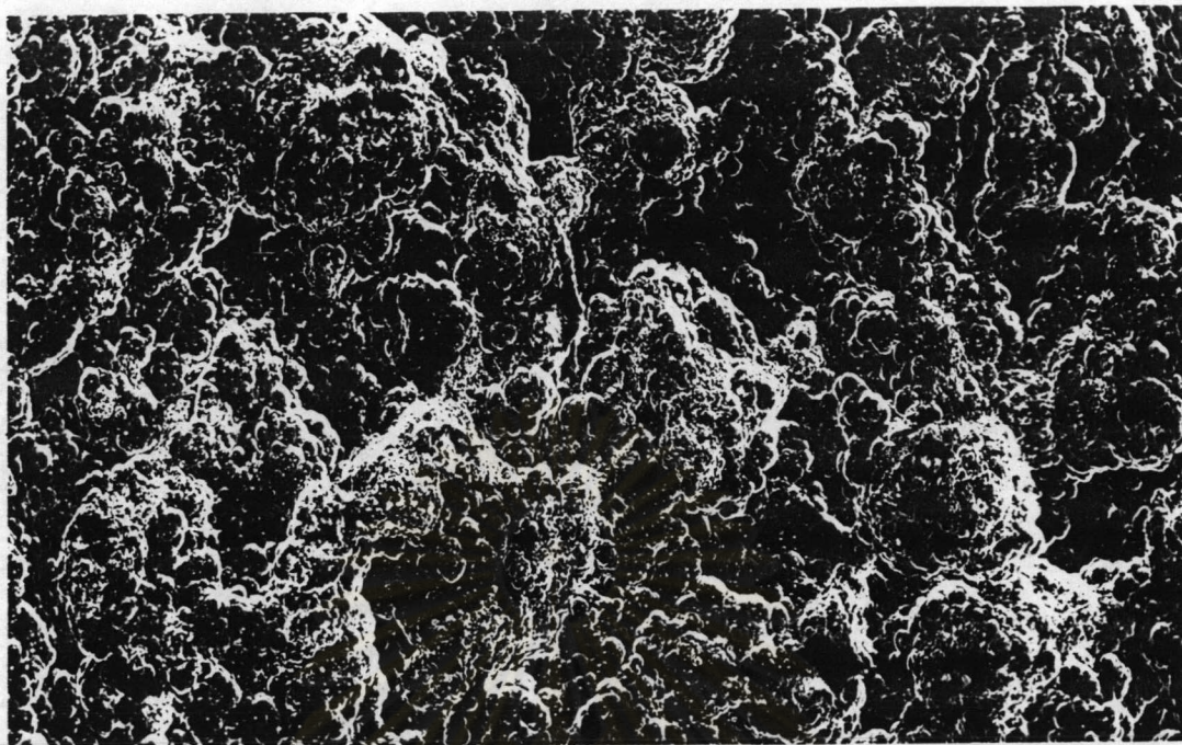
Figure 4.77 SEM photograph with magnification of x60 showing the appearance on surface of the corroded specimens exposed in the \text{CH}_3\text{OH} +saturated \text{H}_2\text{S} +200 ppm DMM solution at ambient temperature for 133 h
