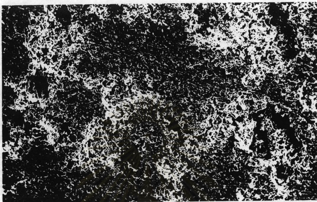
Figure 4.67 SEM photograph with mag. x60 showing the appearance on the same corroded surface immersed in the \text{CH}_3\text{OH}+150 ppm \text{HCl}+150 ppm DMM solution at temperature, lower than 20^\circ\text{C} .
