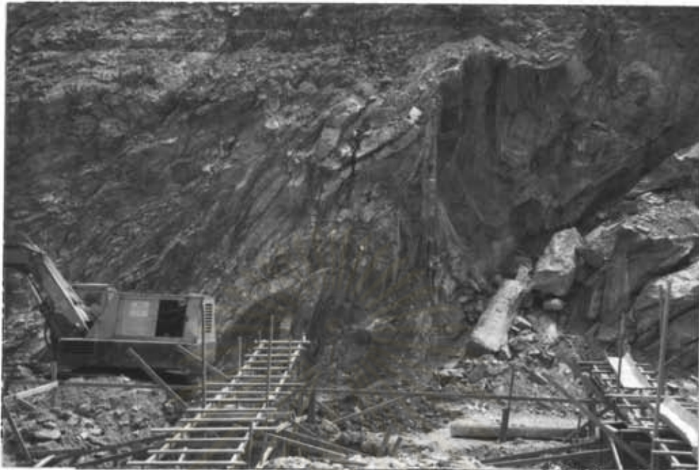
Figure 58 Photograph showing the fault drag at grid reference 25301870, Siam Cement Co. Ltd. Quarry.
