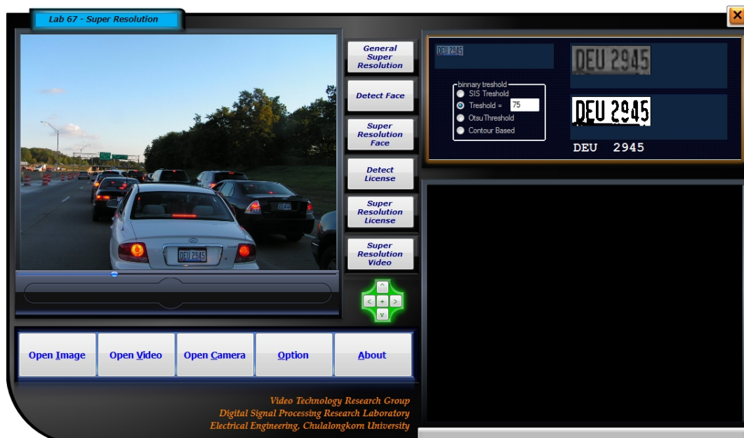
Figure 6.3: Screen shot of license plate super-resolution and license plate recognition.
