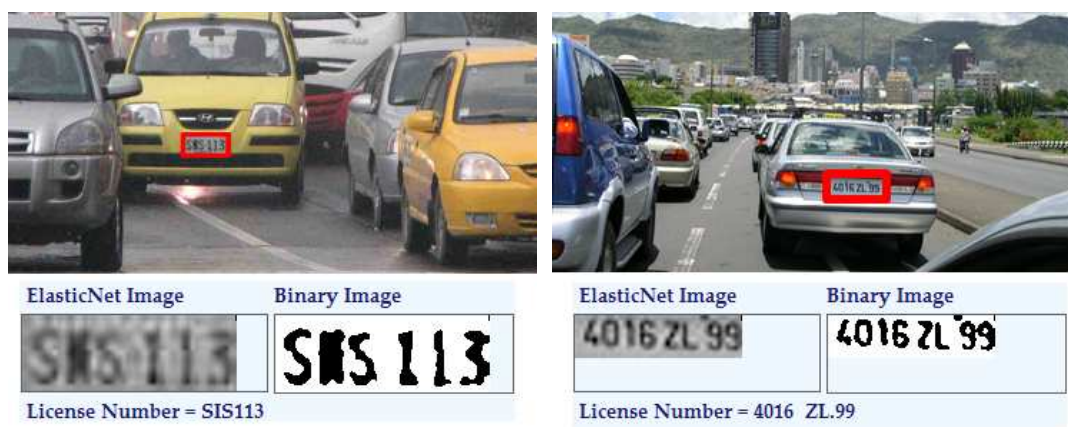
Figure 4.9: Character recognizing on blurry and noisy low resolution license plate images. Low resolution images were upsized using Elastic Net and then converted to binary image. From binary image, license plate number was detected using OCR.
