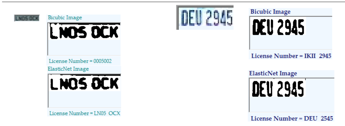
Figure 4.11: Character recognizing on blurry and noisy license plate images. Low resolution images are upsized using bicubic and Elastic Net.
