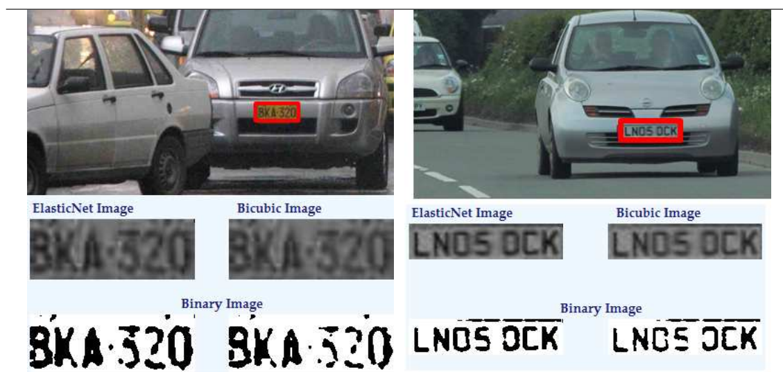
Figure 4.10: Character recognizing from frontal and non-frontal license plate image. Low resolution images are upsized using bicubic and Elasticnet.
