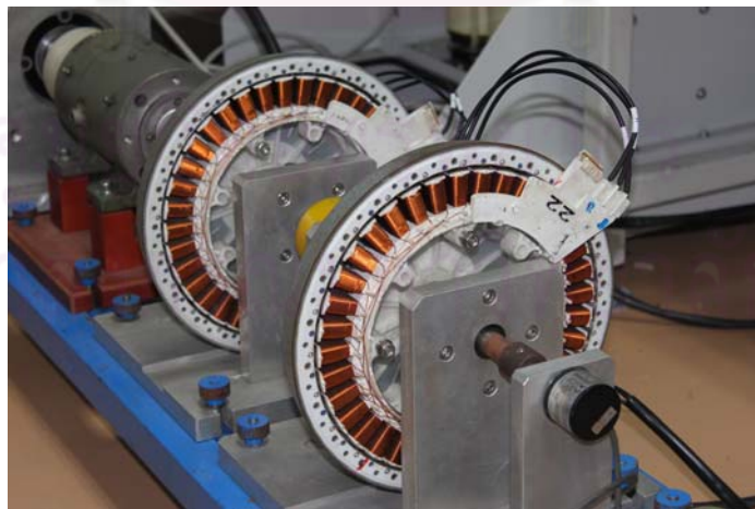
Fig. 2.4 Photo of two synchronous generators arranged in tandem
