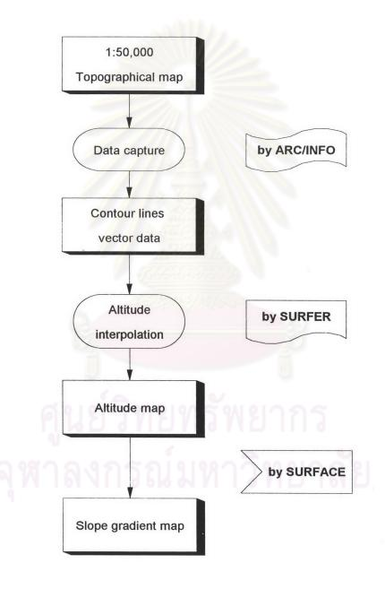
Figure 3.3 The process of slope gradients generation diagram
