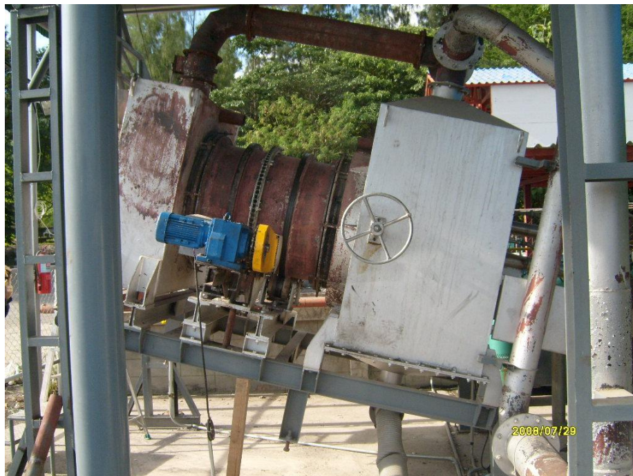
Figure A.2: The pilot-scale rotary cement kiln which can be lifted to remove the clinker inside the kiln
