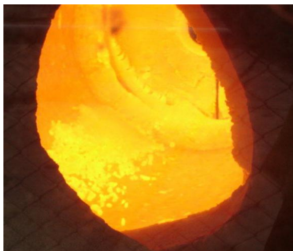
Figure A.7: The sample was burning in the pilot-scale rotary cement kiln
