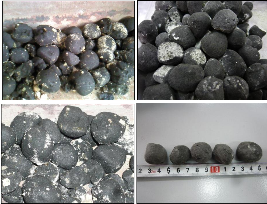
Figure B.8: The clinker after burning by the pilot-scale rotary cement kiln
