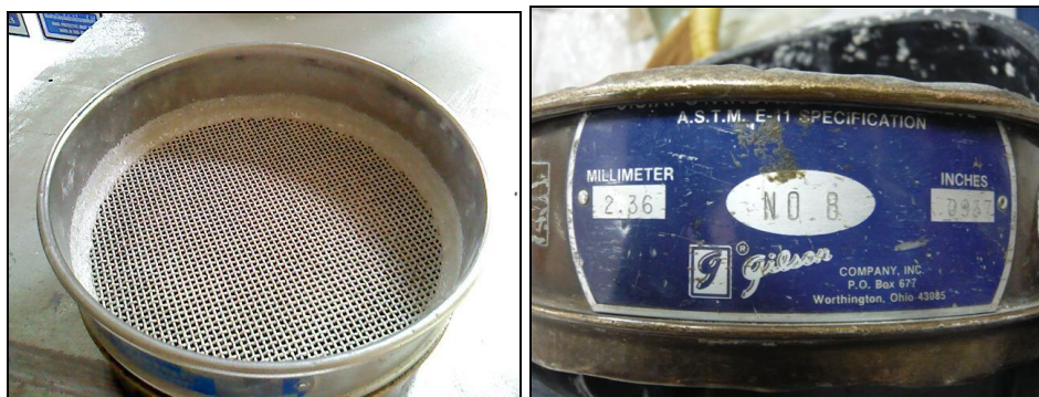
Figure B.13: Sieve no.8, 2.36 millimeters was used to sieve crushed clinker before sending to lab ball mill machine
