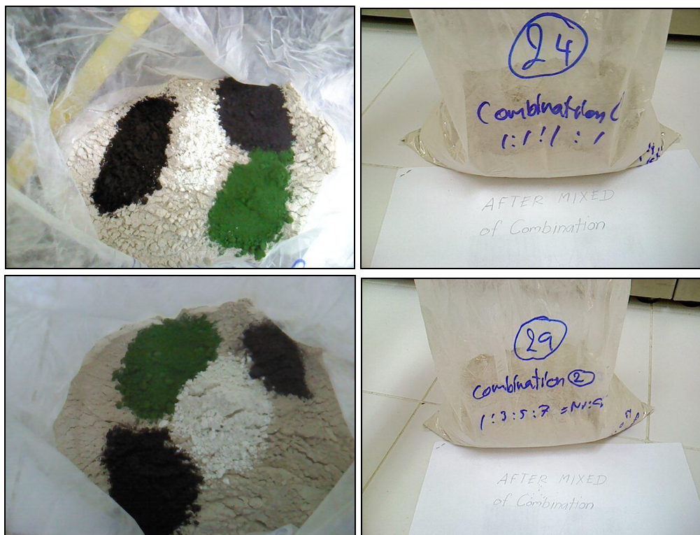
Figure B.6: Examples of kiln feed were added combination of heavy metals
