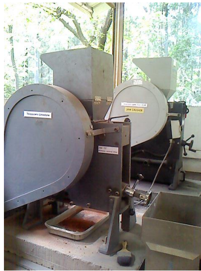
Figure B.12: Jaw crusher for crushing clinker
