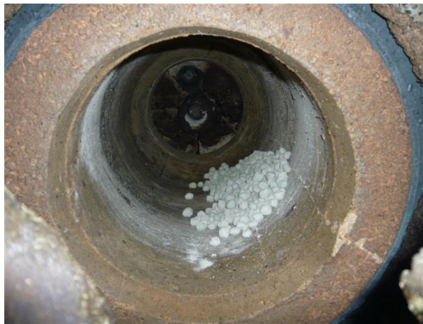
Figure A.6: The sample before burning in the pilot-scale rotary cement kiln
