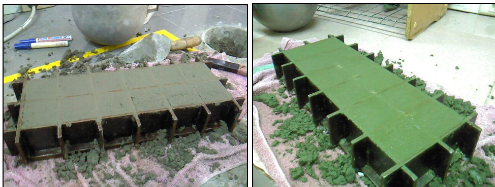
Figure B.16: Cement mortar in the molds
