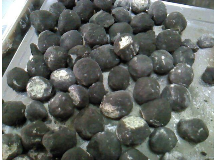
Figure A.8: The clinker after burning in the pilot-scale rotary cement kiln
