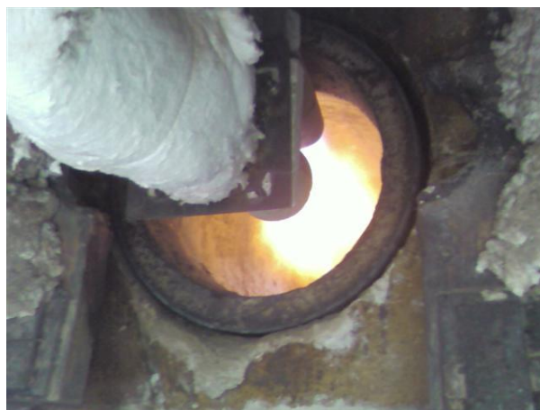
Figure A.4: The two LPG burners were used for heating in the kiln
