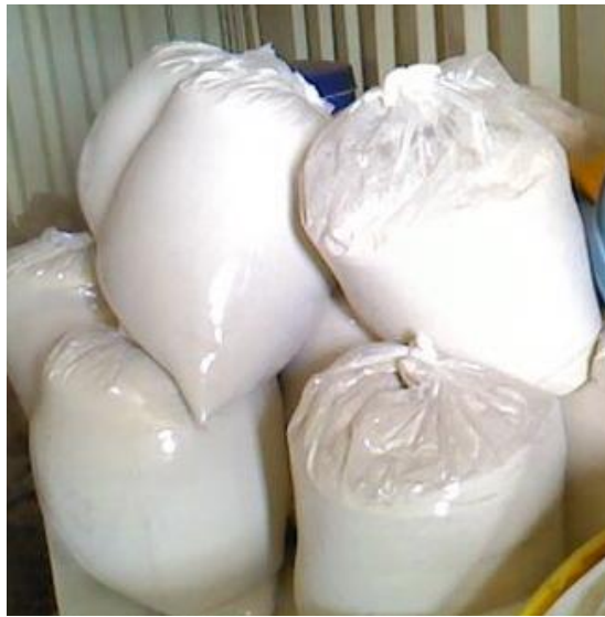
Figure B.5: Kiln feed after pre-calcinations
