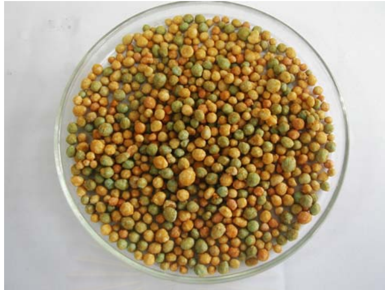
Figure 4.11 Fertilizer coated with 10 pph tung oil by pan coating method.
