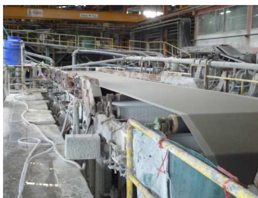
Figure 1 The raw materials have been transformed into sheet through curing process. Wet surfaces causing slips and falls and electrical cables on wet surfaces cause electrocution
