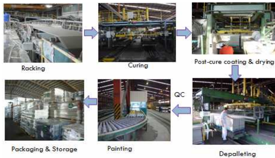
Figure 4.2 Racking, curing, post-cure coating & drying, depalleting, painting and packaging & storage
