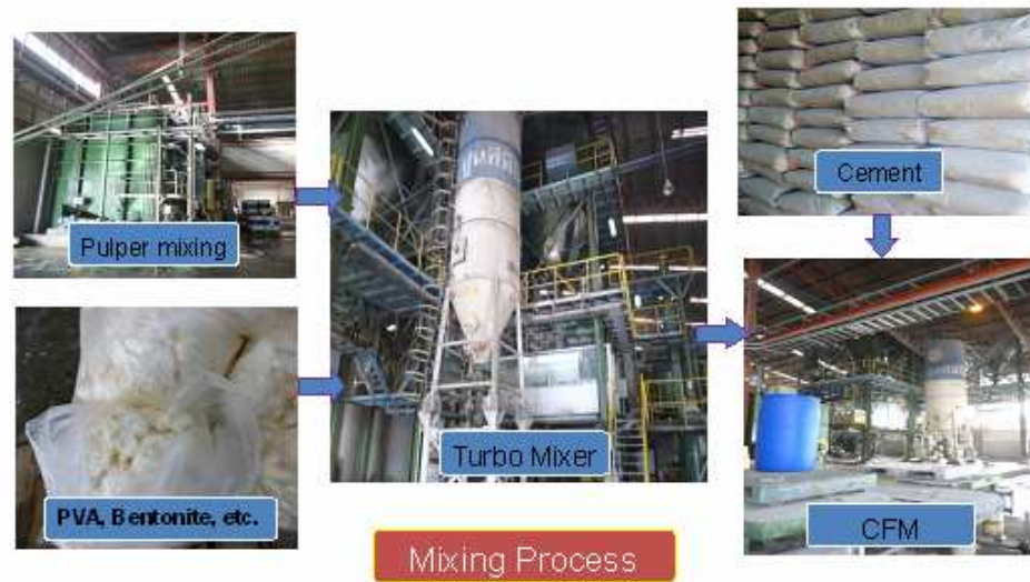
Figure 4.1: Mixing process of fiber cement factory (CFM = centrifuge ingredient mixing)
