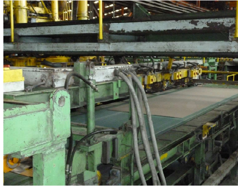
Figure 4.3 Total and respirable dust exposure at de-palleting and skid may cause irritation and inflammation of the eyes, and aggravate pre-existing respiratory symptom conditions.
