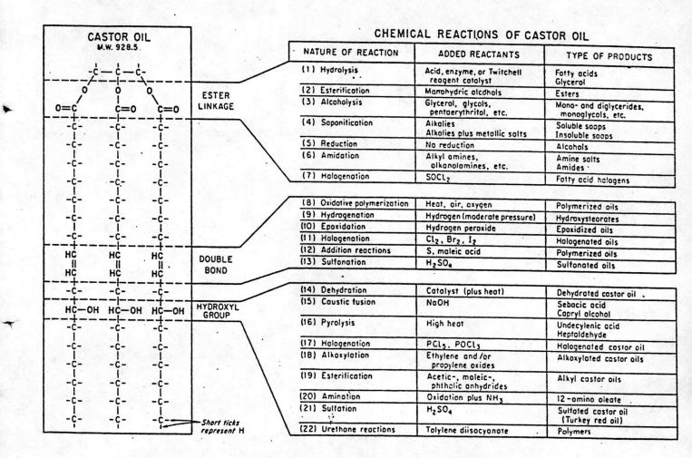
Figure 2.2 Chemical reactions of castor oil
