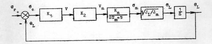
Figure 2.2. Block Diagram with Transfer Functions for Tracking System.
