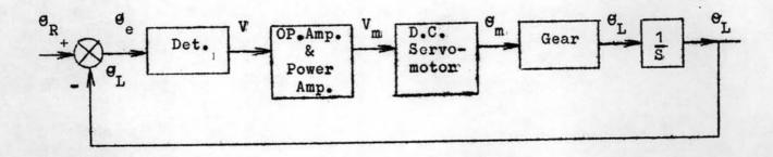
Figure 2.1. Block Diagram of the Tracking System.
