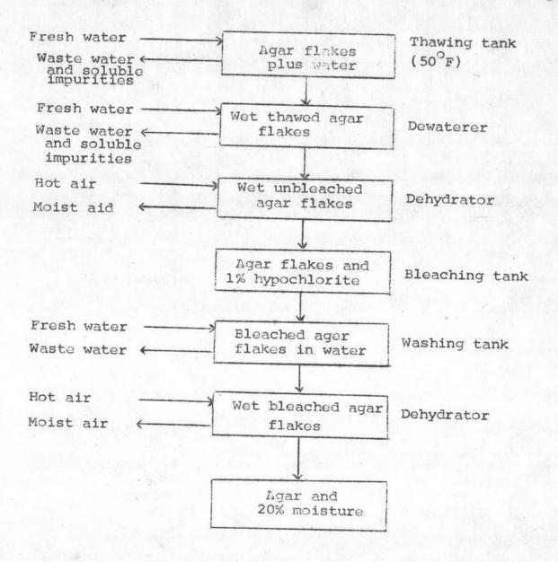
Figure 2-1 Flow diagram of the American process of agar manufacture as used in California. The bleaching portion is used by only one firm.
