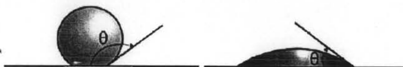
Figure 2.3 Liquid droplet in equilibrium: definition of the contact angle.
