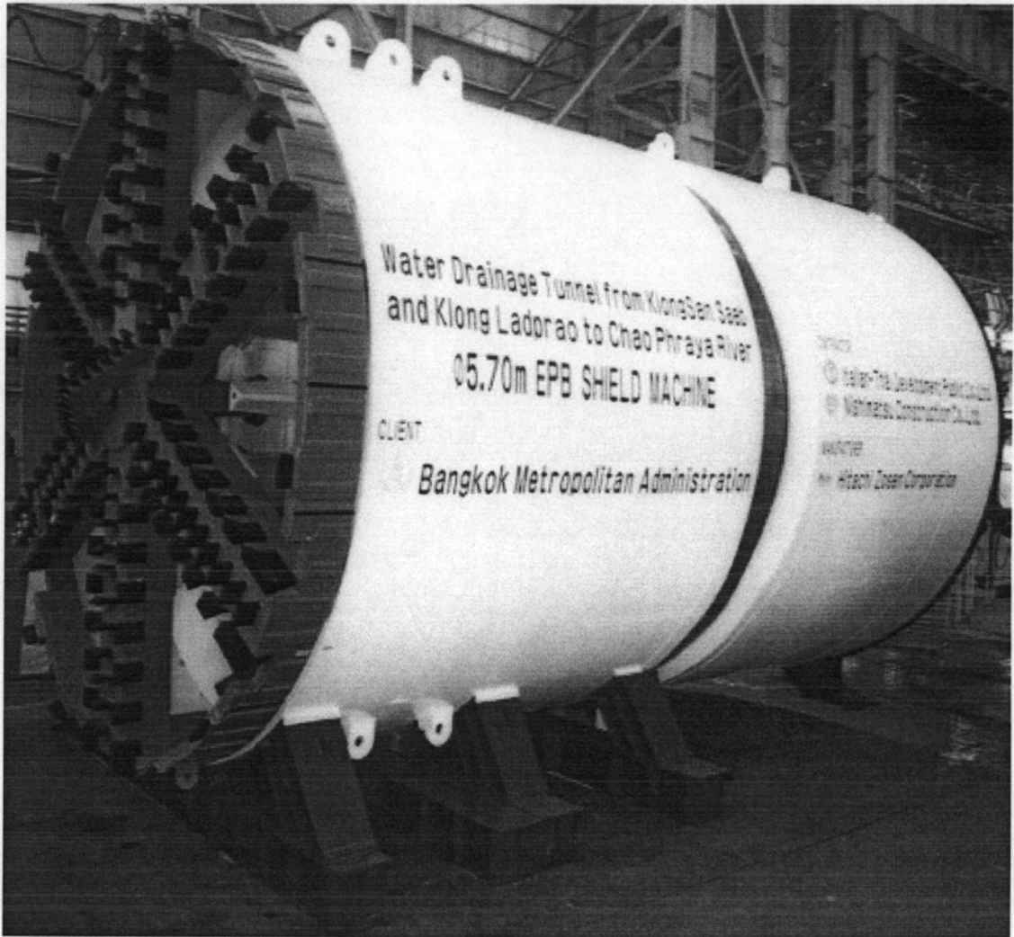
Figure C.1 Articulated EPB shield for MBA flood diversion tunnel (Saensaep-Latphrao Phrakhanong project)
