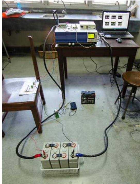
Figure 5-9 Configuration of electronic load and lithium-ion batteries on the test-bench
