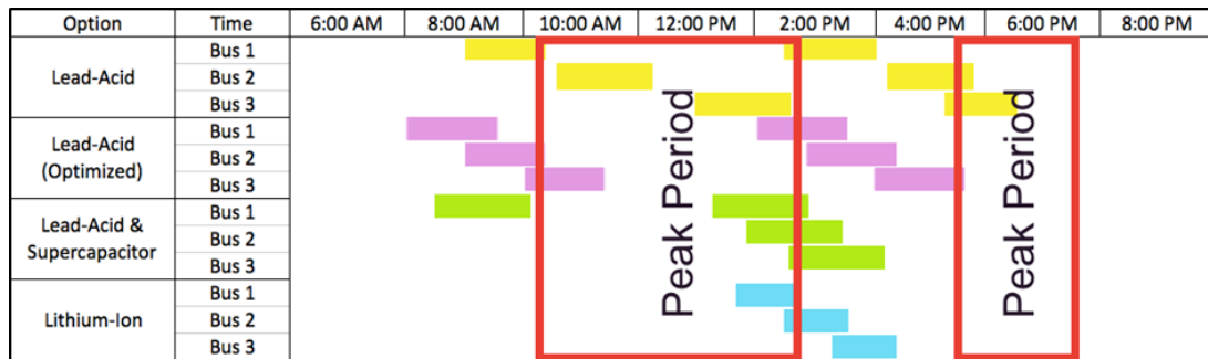
Figure 6-1 Bus charging time schedules for three types of energy storage
