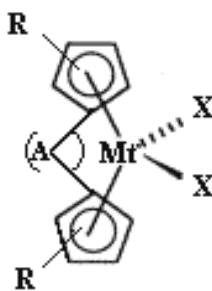
Figure 2.1. Typical chemical structure of a metallocene catalyst [where Mt is the transition metal, normally from Group 4, 5, or 6 e.g. Zr, Ti or Hf, A is an optional bridging unit consisting of 1-3 atoms in the backbone, R is hydrocarbyl substituents or fused ring systems (indenyl, fluorenyl and substituted derivatives) and X is chlorine or other halogens from group 7 or an alkyl group] (Alt, 1999).
