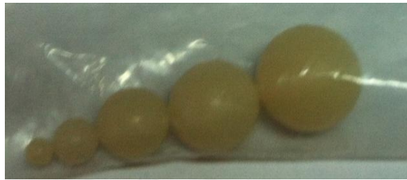
Figure 3. 3 Simulated lung nodule of sphere 12, 10, 8, 5 and 3 mm in diameters
