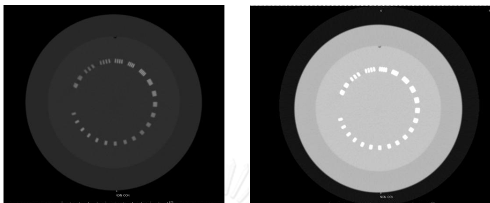
Figure 4. 6 Spatial resolution part of Catphan phantom
