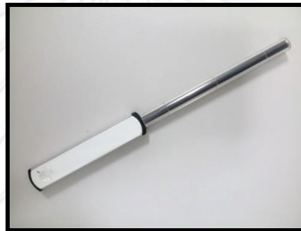
Figure 3.6: Pencil ionization chamber: Unfors Xi CT detector
