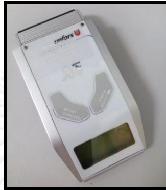
Figure 3.8: Unfors Xi base unit with mAs display
