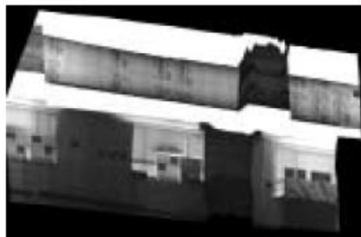
รูปที่ 3.5 The 3-D geometric model and the geometric model plus texture maps (El-Hakim et al. 1997)
