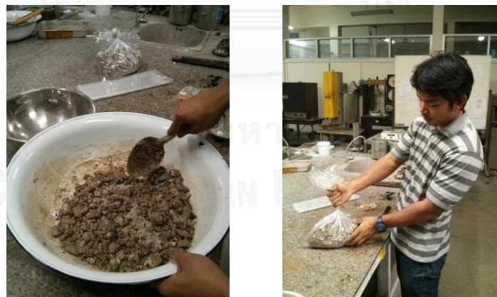
Figure 4.2 Mixing Aggregate with Water and Storing in Plastic Bag
