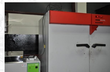
Figure 4.7 Oven Setup for Controlling Laboratory Sample Temperature
