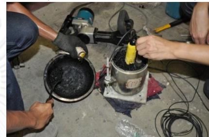
Figure 4.5 Insertion of Thetaprobe into Compacted Laboratory Sample
