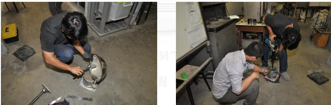
Figure 4.4 Compaction of Laboratory Sample for Temperature Verification
