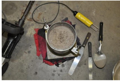
Figure 4.5 Insertion of Thetaprobe into Compacted Laboratory Sample
