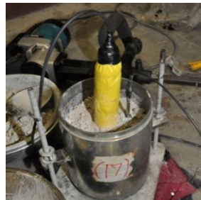
Figure 4.5 Insertion of Thetaprobe into Compacted Laboratory Sample
