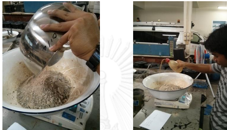
Figure 4.1 Aggregate and Water Weight Measurement
