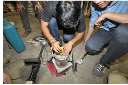
Figure 4.5 Insertion of Thetaprobe into Compacted Laboratory Sample
