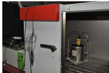
Figure 4.7 Oven Setup for Controlling Laboratory Sample Temperature
