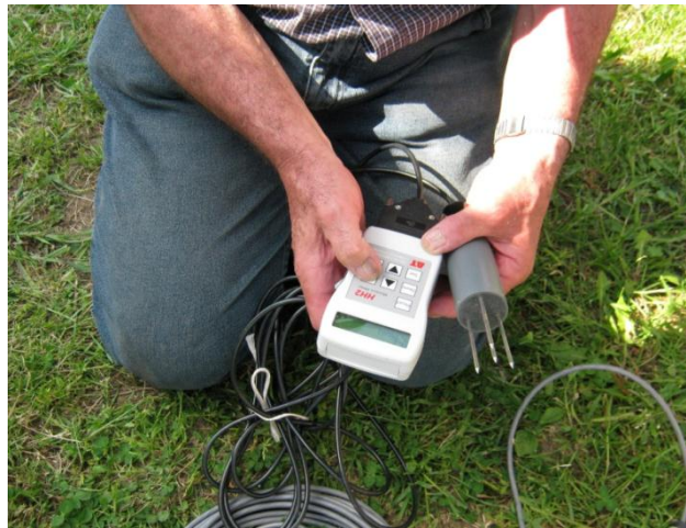
Figure 3.10 ML2x-Thetaprobe in the Field source: hydropedologie.agrobiologie.cz
