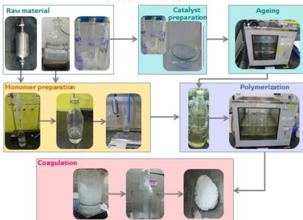
Figure 2.3 Flow diagram of screening test for BD polymerization.
