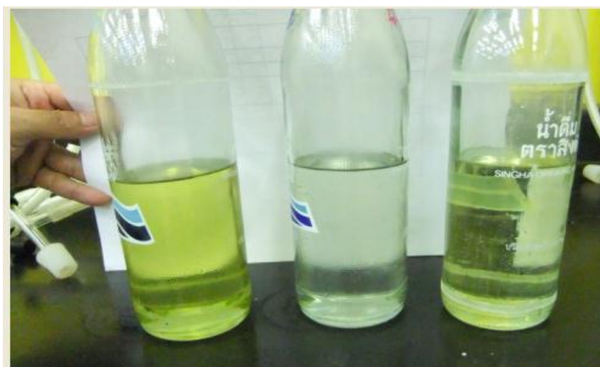
Figure 3.3 No reaction occurred in the BD polymerization using \text{NdV}_3/\text{DEAC} .
