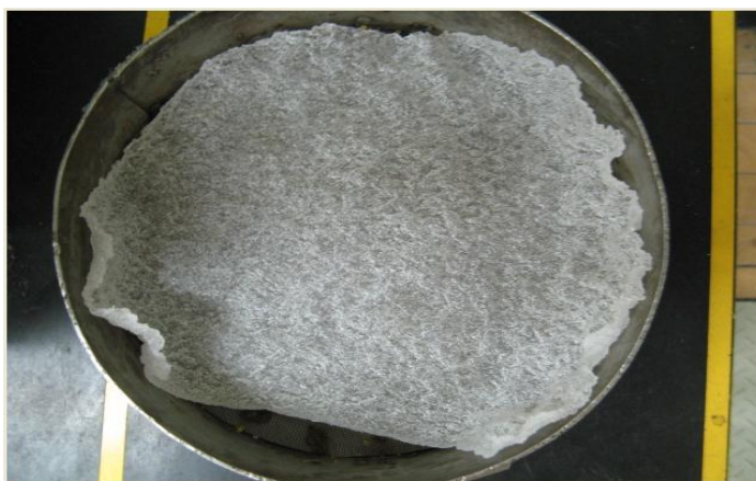
Figure 2.2 BR products after drying at 80 °C.
