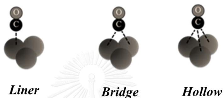
Figure 25 Model of CO adsorption behaviors
