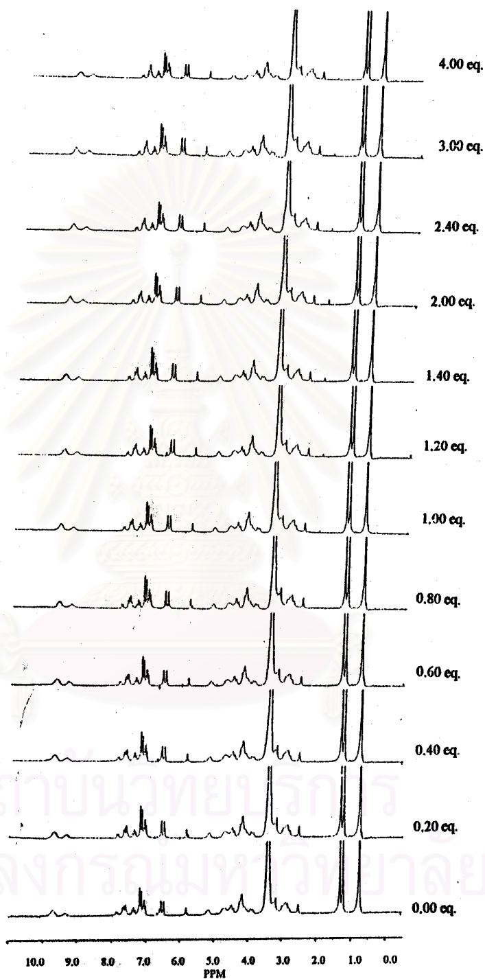
Figure C.2 1 H-NMR (DMSO- d 6 ) spectra of complexation between 6a and NaNO 3 at 0:00-4:00 ratios.
