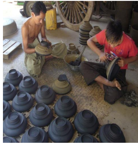
2. Coating many layers with resin (Thit-si inyanmar)
