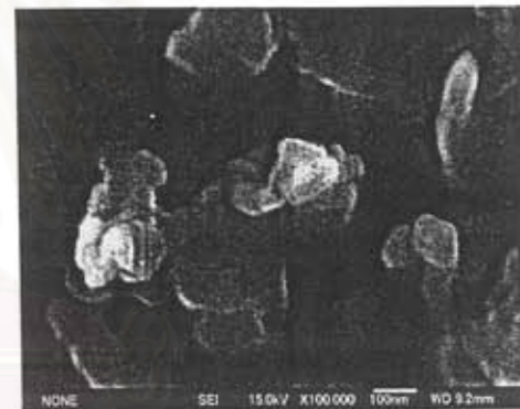
Fig. 3. Surface morphology by 10^5 \times FE-SEM as a function of the MgO buffer layer thickness: (a) 0 nm, (b) 145 nm, and (c) 300 nm.
