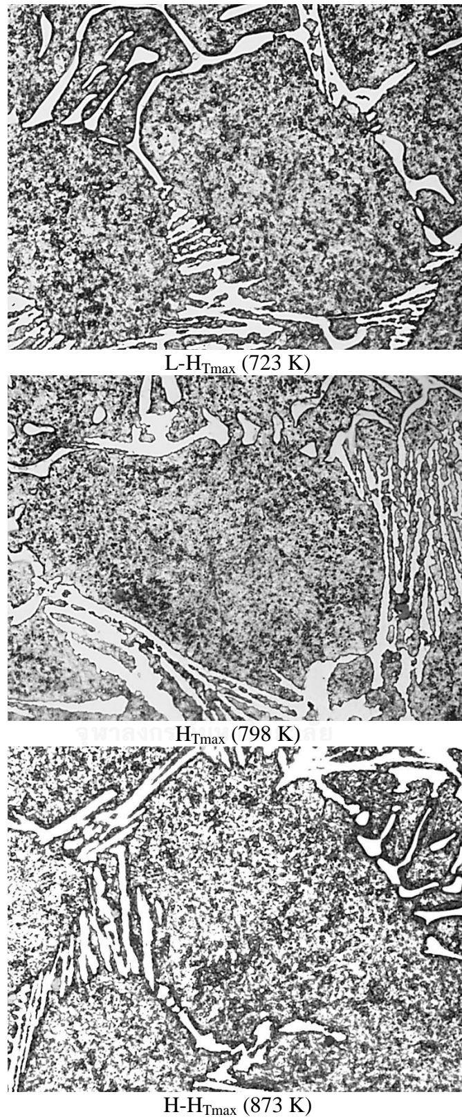
Fig. 4-10 Comparison of microstructures of L-H_{T_{max}} , H_{T_{max}} and H-H_{T_{max}} specimens in No.2 with 2.00% C tempered after hardening from 1323 K austenitizing.
