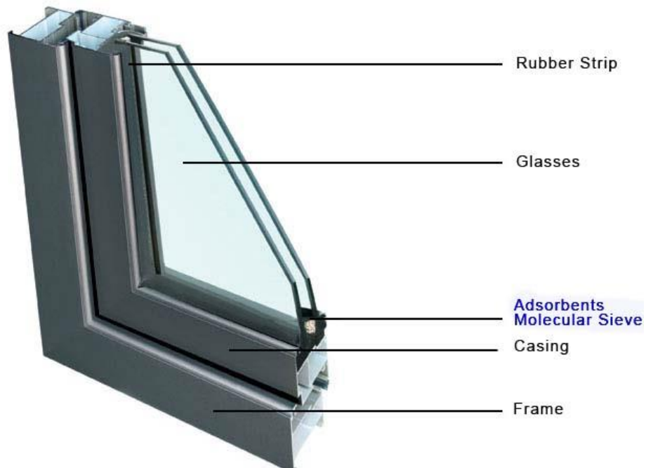
Figure a - 4 Insulated Glass.
