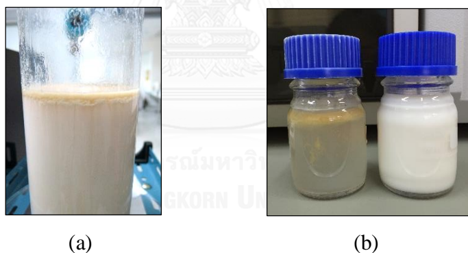
Figure 4.10 Emulsion appearance after \text{CaCl}_2 addition (1% w/v): (a) during process; (b) left: over night settling; right: a sample suddenly collected from the process
