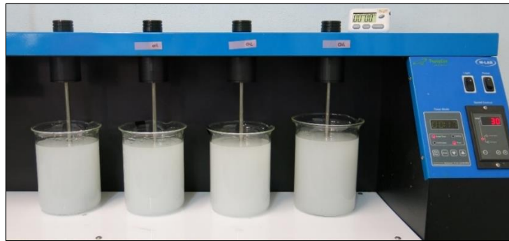
Figure 3.17 Experimental setup of the jar-test technique
