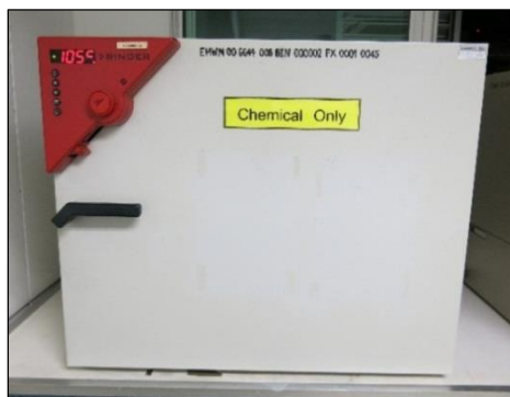
Figure 3.9 An oven used for water evaporation
