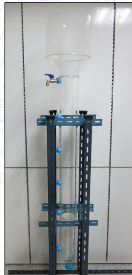
Figure 3.3 The configuration of coalescer column
