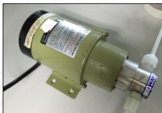
Figure 3.7 The magnetic gear pump used in cross-flow UF
