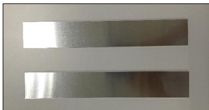
Figure 3.12 Electrode plates made of Al
