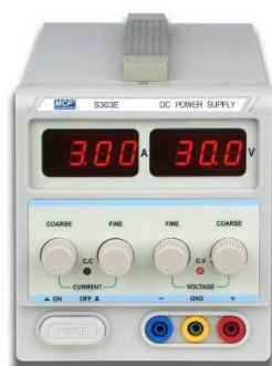
Figure 3.11 A DC power supply machine
