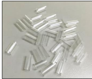
Figure 3.4 The tubular coalescing media
