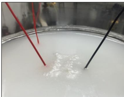
Figure 4.28 The hydrogen gas ( H_2 ) taking place during the electrocoalescence
