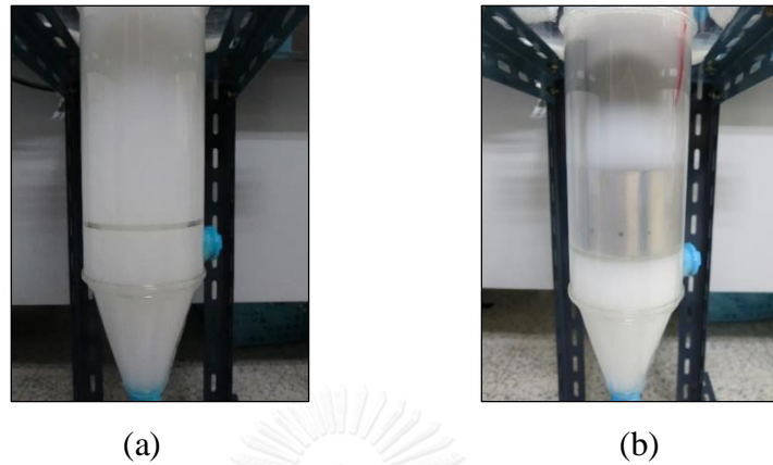
Figure 4.5 Experimental setup of the (a) decantation and (b) coalescer
