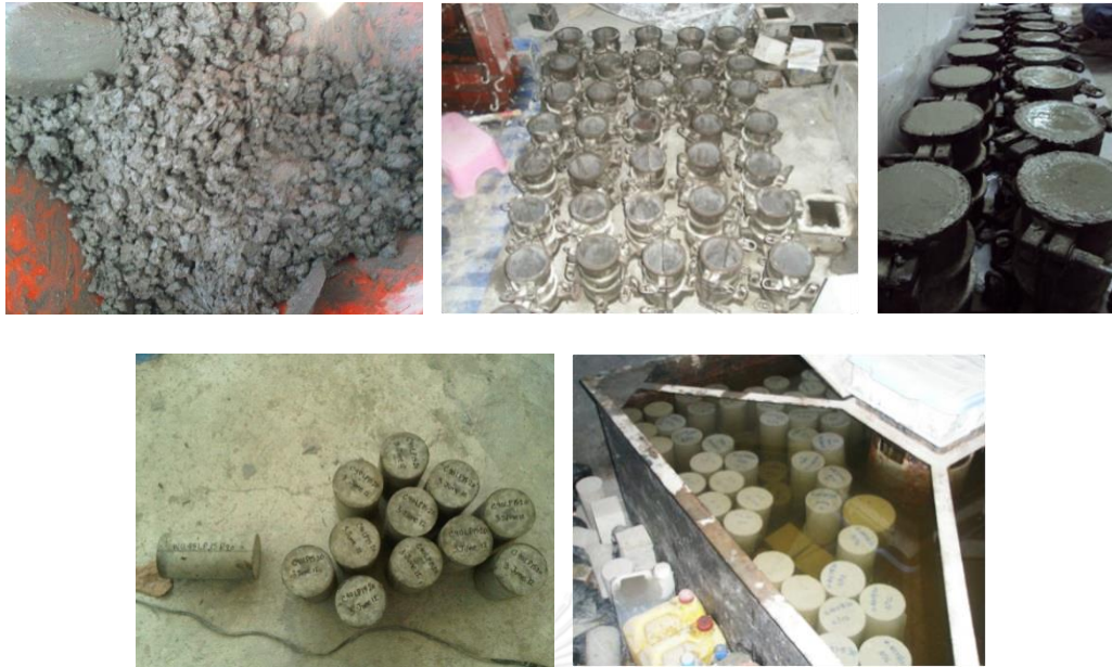
Figure 3.2 Concrete sample preparation
