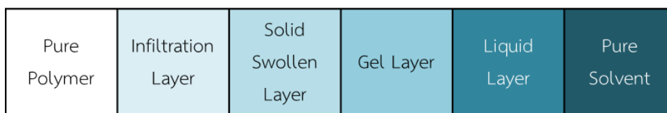
Figure 4.9. Schematic picture of the composition of the surface layer [75].
