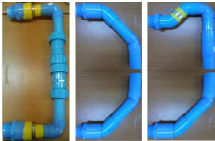
Figure 4.13 Example of downcomer with 1.5 inches diameter
