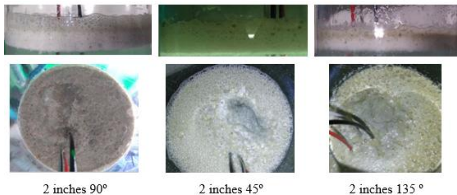
Figure 4.18 Sludge generation in different connector configuration at 100 cm 1.5 g/l
