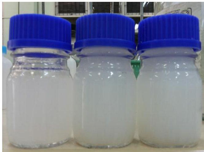
Figure 4.1 Synthetic cutting-oily wastewater at different concentrations (left) 0.5 g/l (middle) 1.0 g/l (right) 1.5 g/l
