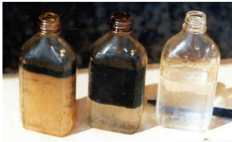
Figure 2.3 The effluent at the top and bottom outlet ("Produced water treatment," 2014) (left) influent, (middle) oil from the top outlet , (right) effluent from the bottom outlet
