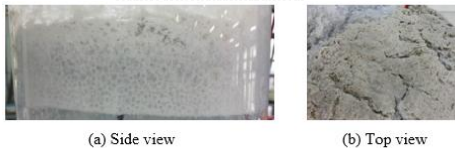
Figure 4.23 Sludge in reactive and stabilizing stage
