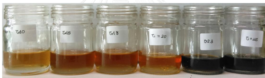
Figure 5.5. Biofuel samples from RPO under SCM conditions at 400 °C, 15 MPa, and a molar ratio of 12:1 at different residence times. The sequence of vials from left to right is residence times of 10, 15, 18, 20, 23, and 25 min, respectively.
