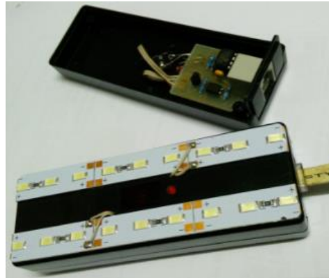
Figure 31 LED driver and circuit inside
