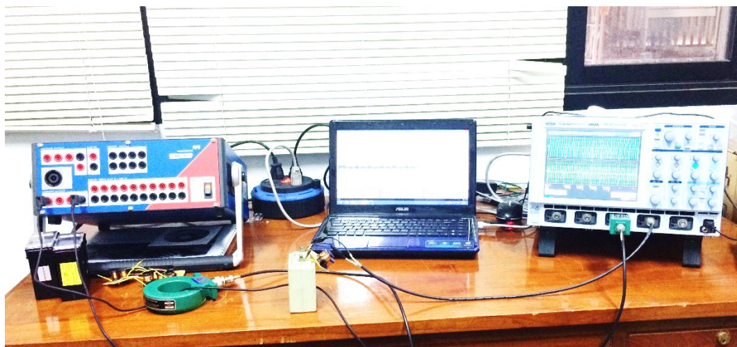
Figure 3-16: Real test circuit when harmonic current was injected to CT2 with standard burden C.
