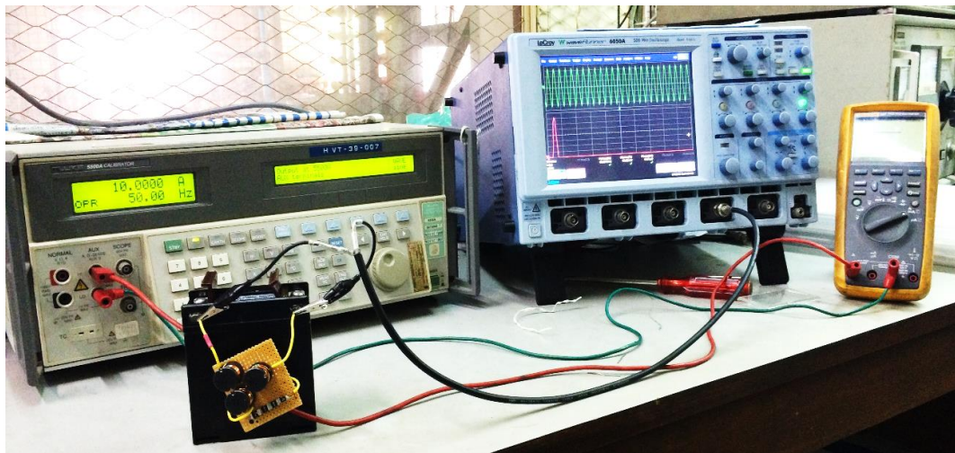
Figure 3-10: Real test circuit when single frequency current was injected to CT1 with standard burden B.
