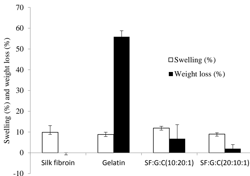
Figure 26 Weight loss and swelling of SF, G, and SF: G: C at 10:20:1 and 20:10:1 nanofiber mats after crosslinking with ethanol
