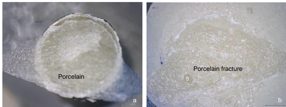
Figure 20 Cohesive failure in porcelain: (a) restorative site, (b) porcelain site (BF group)
