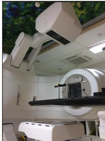
Figure 3. 22 The setup for incident air kerma measurement from OBI system
