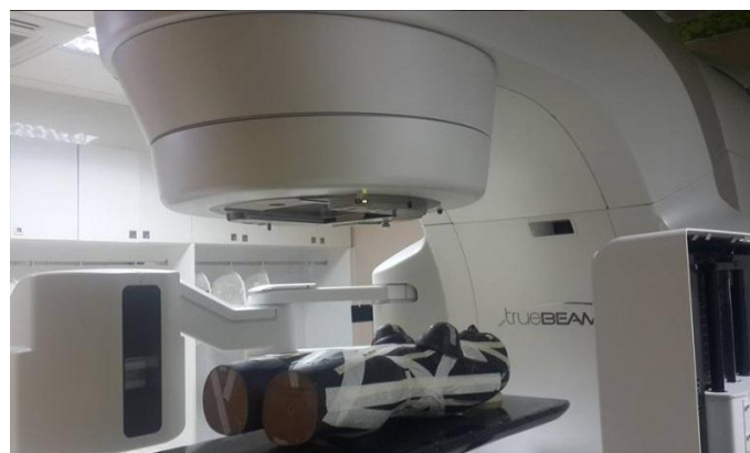
Figure 3. 24 The setup of RANDO phantom to scan the CBCT pelvic protocol
