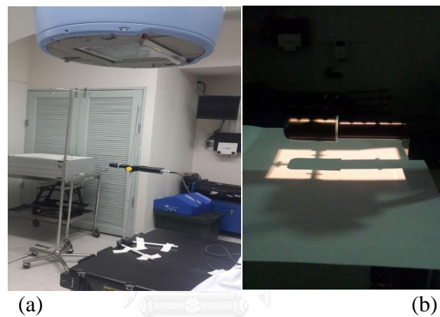
Figure 3. 18 (a) Chamber setup (b) field size opened just to cover the chamber to avoid backscatter for Incident Air Kerma measurement
