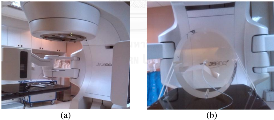
Figure 3. 23 The 100cc pencil chamber (a) at the isocenter in air and (b) in the PMMA body phantom for CBDI measurement
