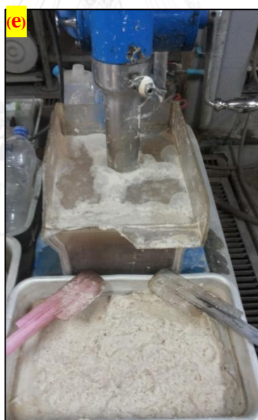
Figure 3. 11 (a, b, c, d and e) Equipment, reagents and procedure of Froth flotation method
