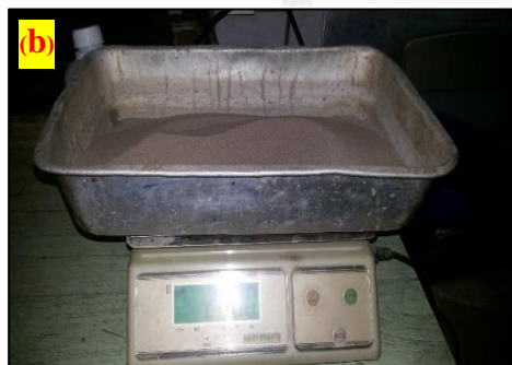
Sample weighted in the tray with electronic balance
