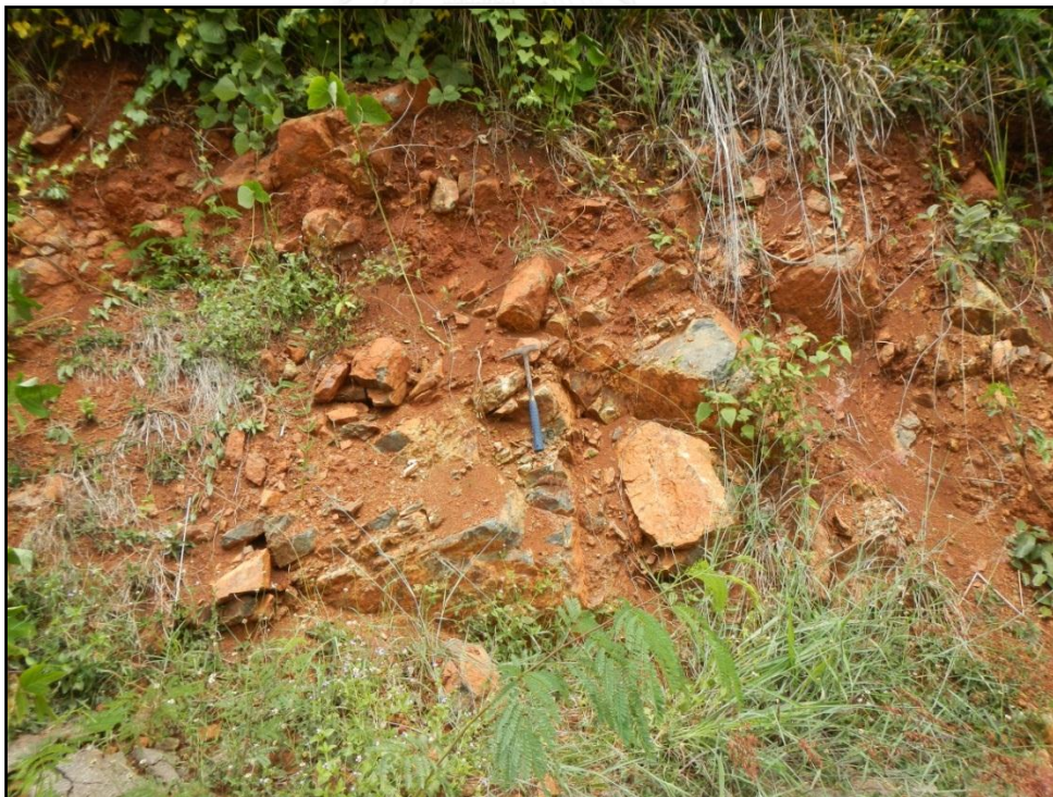
Figure 3.59 Photograph hornblende granite outcrop ID13 (Looking to SW) foliation plane 097^{\circ}/33^{\circ} dip direction to SW. Coordinate 794498E/1599317N.
