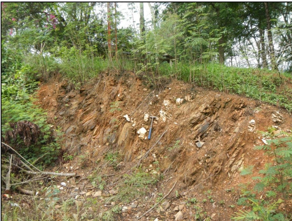
Figure 3.4 Photograph shows outcrop ID44 of shale (Looking to SW) illustrates bedding plane 038^{\circ}/64^{\circ} dip direction to SE. Coordinate 787959E/1611504N .
