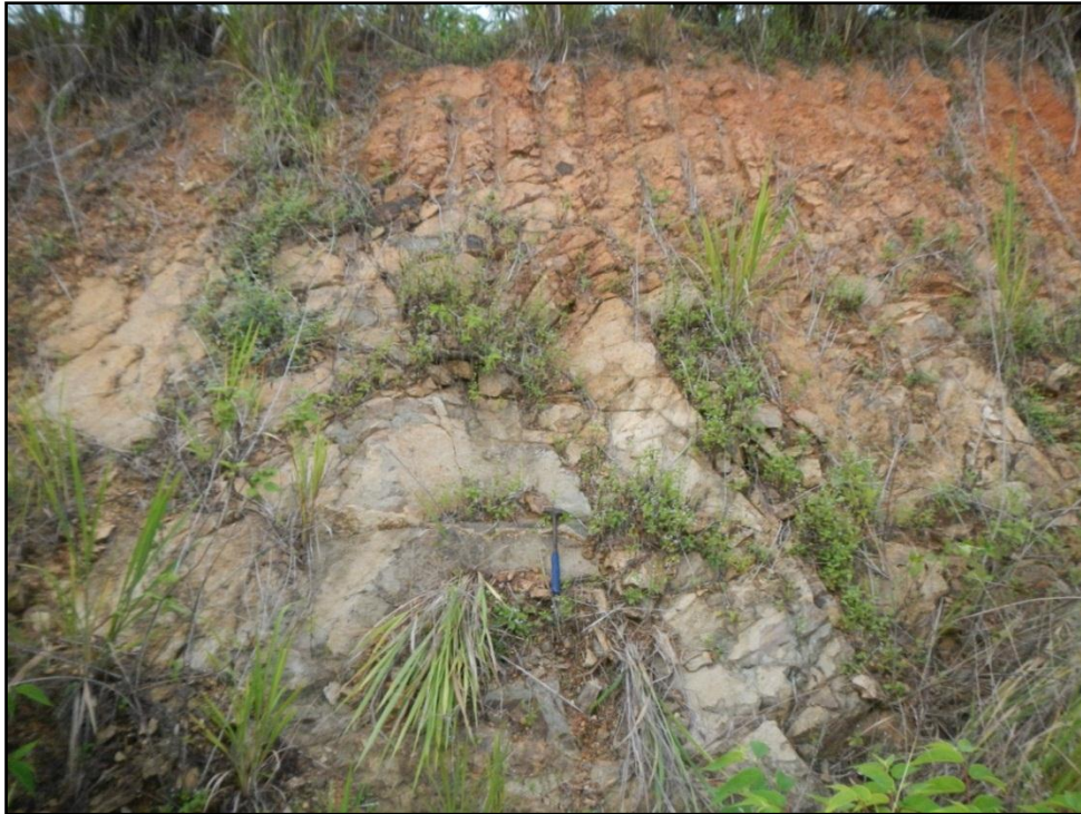
Figure 3.30 Photograph tuff outcrop ID32 (Looking to S) orientation 066^{\circ}/63^{\circ} dip direction to NW. Coordinate 805302E/1594530N.
