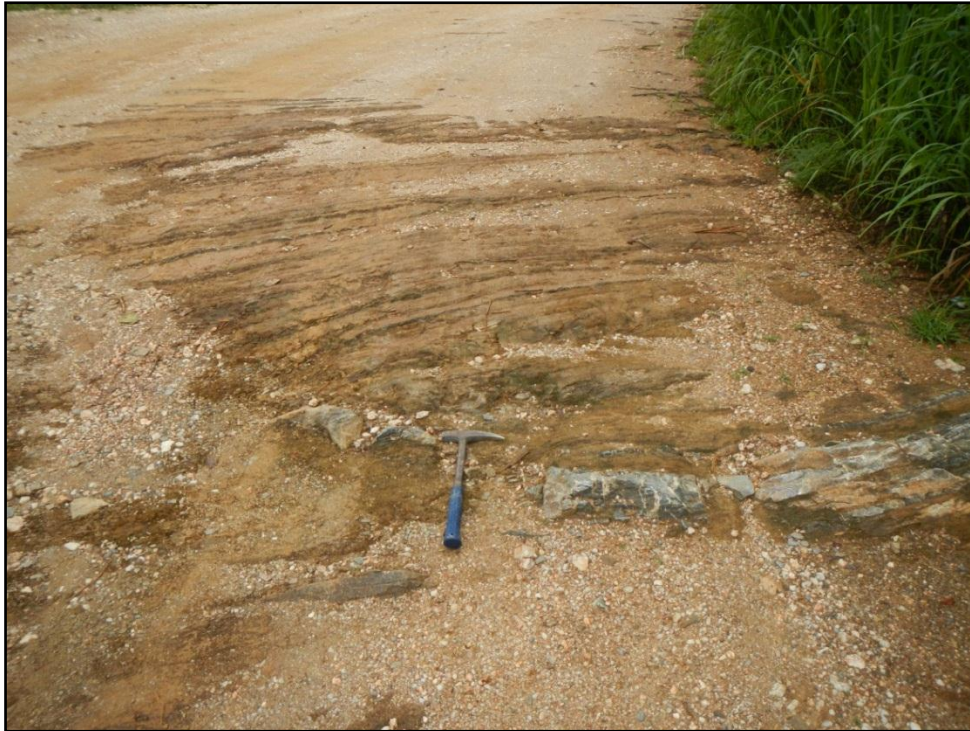
Figure 3.14 Photograph shows outcrop of siltstone interbedded limestone ID43 (Looking to SE) bedding plane 022^{\circ}/38^{\circ} dip direction to SE. Coordinate 789830E/1609385N.
