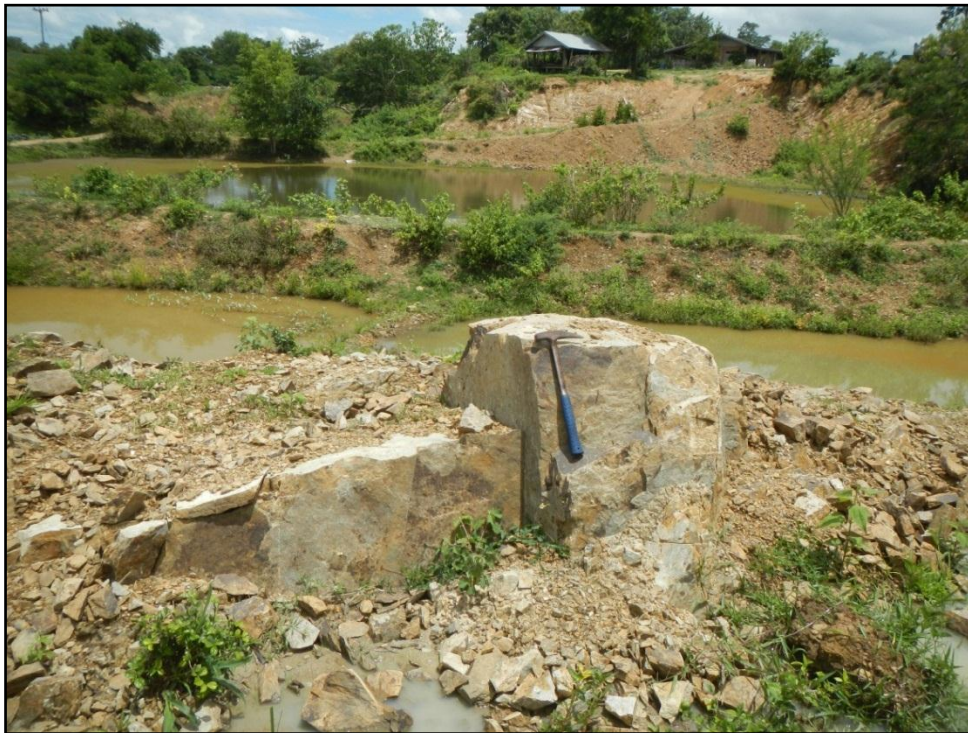
Figure 3.29 Photograph of tuff outcrop ID4 (Looking to S) orientation 262^{\circ}/72^{\circ} dip direction to NW. Coordinate 798106E/1601526N.
