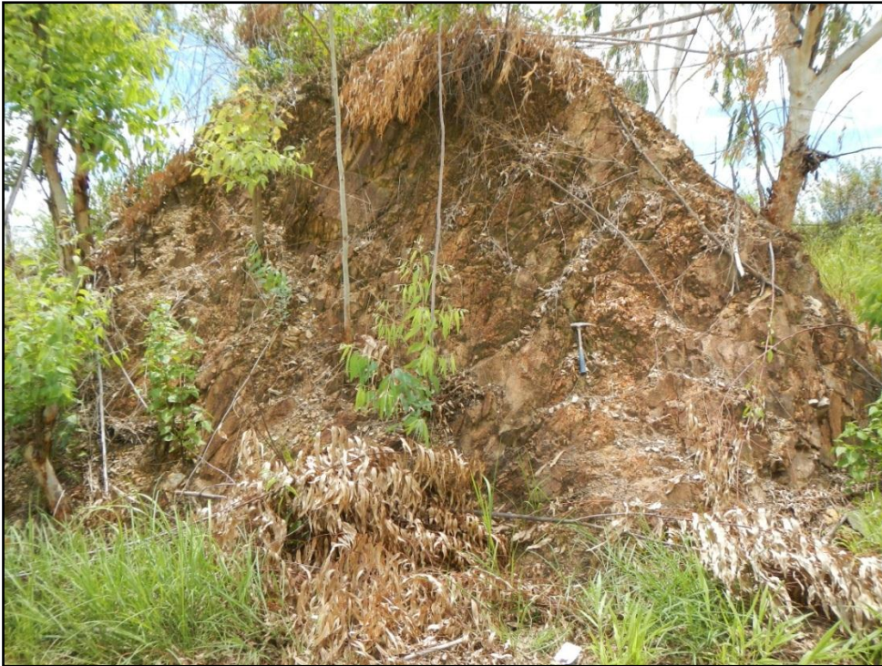
Figure 3.3 Photograph shows outcrop ID12 of siltstone (Looking to E) foliation plane 267^{\circ}/68^{\circ} , dip direction to NW. Coordinate 795544E/1593082N . Hammer has length 16.5 inches.
