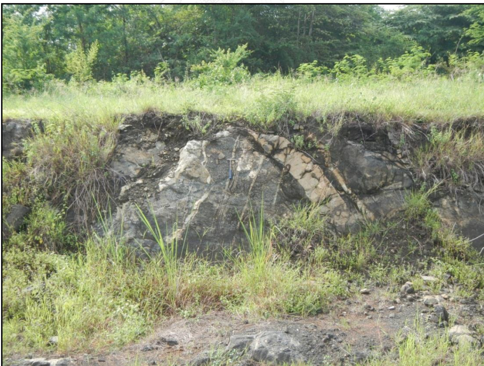
Figure 3.62 Photograph of hornblende granite in abandon mine ID28 (Looking to SE) foliation plane 105^{\circ}/63^{\circ} dip direction to SW. Coordinate 796216E/ 1600554N.
