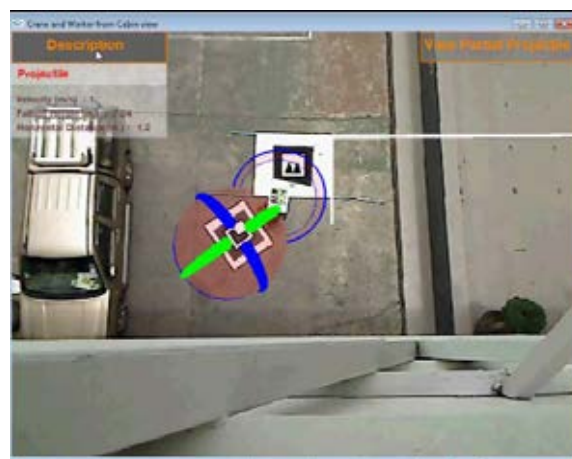
Figure 7.45 The output screen of situation number 4 for verifying the function to illustrate the unsafe working area
