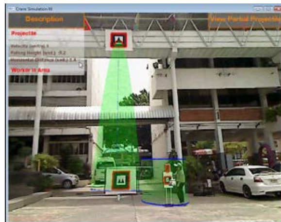
Figure 7.42 The output screen of situation number 1 for verifying the function to illustrate the unsafe working area
