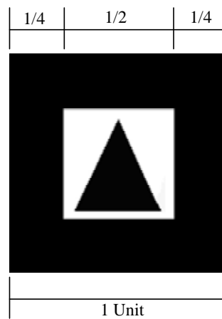
Figure 5.8 Example marker size and pattern
