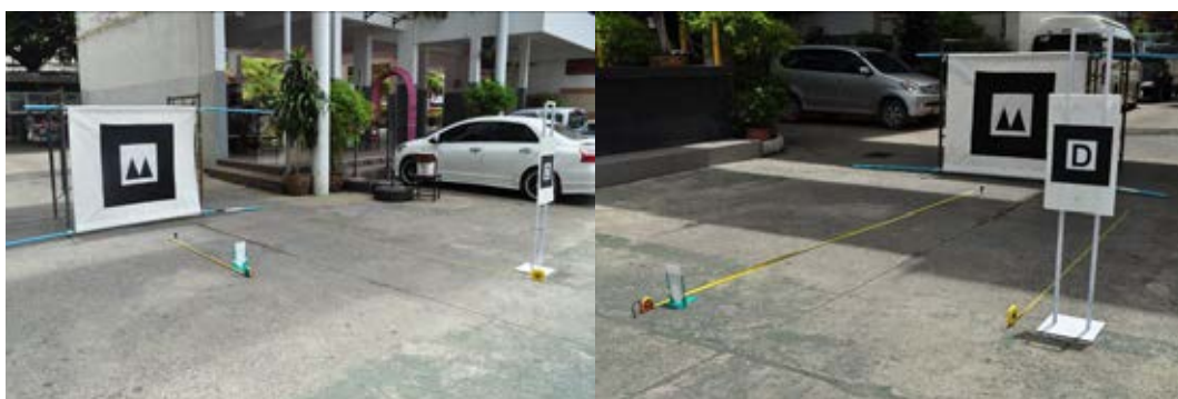
Figure 7.40 Tape measurement in real environment testing
