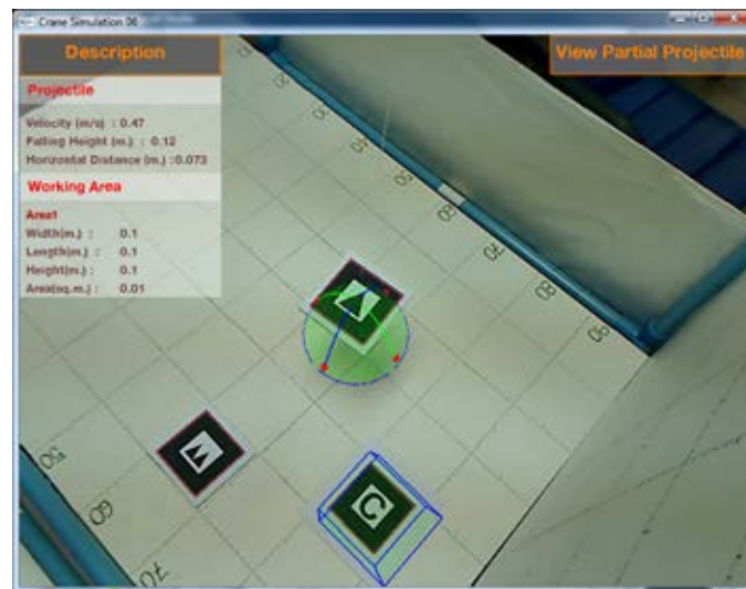
Figure 6.20 Example of output window for hazard of falling object from crane into work area (camera installed above base level)
