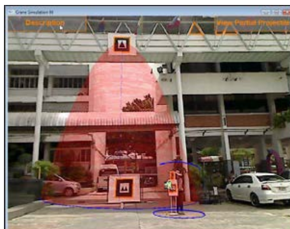
Figure 7.43 The output screen of situation number 2 for verifying the function to illustrate the unsafe working area
