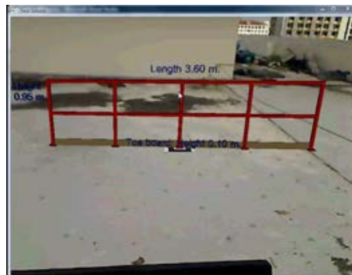
Figure 7.49 Example of 3D virtual guardrail with toe board
