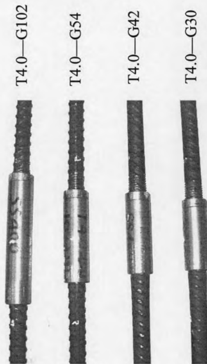
Figure 3.16 Sample of specimens subjected to compression test
