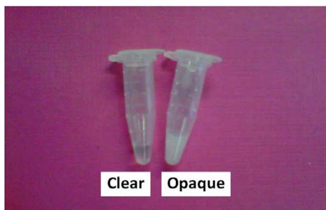
Figure A1 The technique determines the accuracy of the solution. All of solutions, PDADMAC, PSS and PSS-co-MA are clear. PDADMAC is positively charged and the others are negatively charged. When mix between PDADMAC and PSS or between PDADMAC and PSS-co-MA, solutions are opaque.
