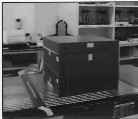
Figure 3.11 Solid water phantom used for dose measurements with EDR2 film
