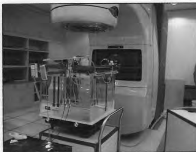
Figure 3.12 Blue phantom with 0.13 cm 2 ionization chamber for depth dose and beam profile measurement
