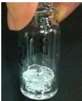
Figure 4.11 A Photograph of PLLA-diMeth gel after immersed in chloroform for 24 h
