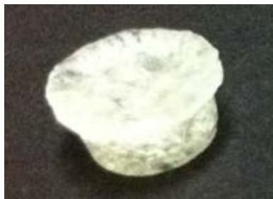
Figure 4.10 Photographs of PLLA-diMeth after thermal crosslinking
