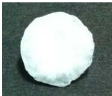
Figure 4.12 Photographs of PLLA-diMeth after UV crosslinking
