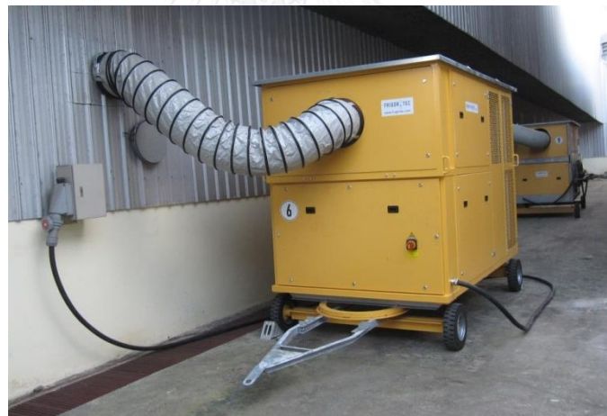
Figure 13 Example of grain cooling unit method
