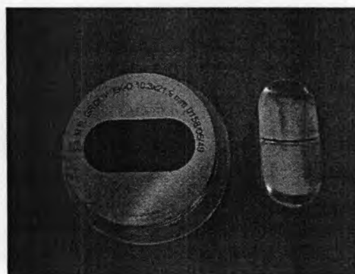
Figure 9 The concaved oblong 10.3x21.9 mm punch and die.
