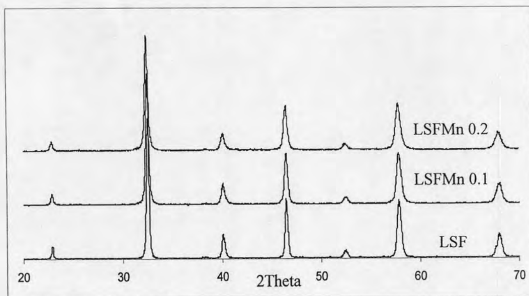
Figure 3.5 XRD pattern of \text{La}_{0.7}\text{Sr}_{0.3}\text{Fe}_{1-x}\text{Mn}_x\text{O}_3 ( x = 0, 0.1 and 0.2 ) powders after calcined at 1000^\circ\text{C} for 6 hours.
