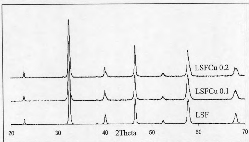
Figure 3.2 XRD patterns of \text{La}_{0.7}\text{Sr}_{0.3}\text{Fe}_{1-x}\text{Cu}_x\text{O}_3 ( x=0, 0.1 and 0.2 ) powders after calcined at 900\text{-}1000^\circ\text{C} for 6 hours.
