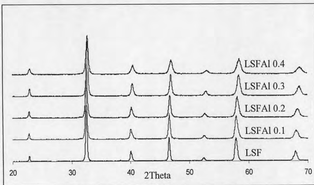
Figure 3.4 XRD pattern of \text{La}_{0.7}\text{Sr}_{0.3}\text{Fe}_{1-x}\text{Al}_x\text{O}_3 ( x=0, 0.1, 0.2, 0.3 and 0.4 ) powders after calcined at 1000^\circ\text{C} for 6 hours.
