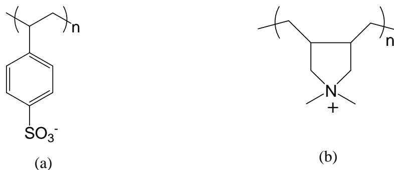
Figure 2.3 Structure of (A) PSS as an anionic polyelectrolyte and (B) PDADMAC as a cationic polyelectrolyte.
