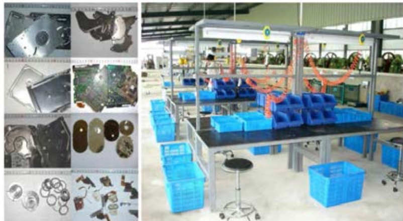
Figure 2-10: manual dismantling of hard disks (left) and dismantling table with pneumatic tools (right) (StEP, 2009)
